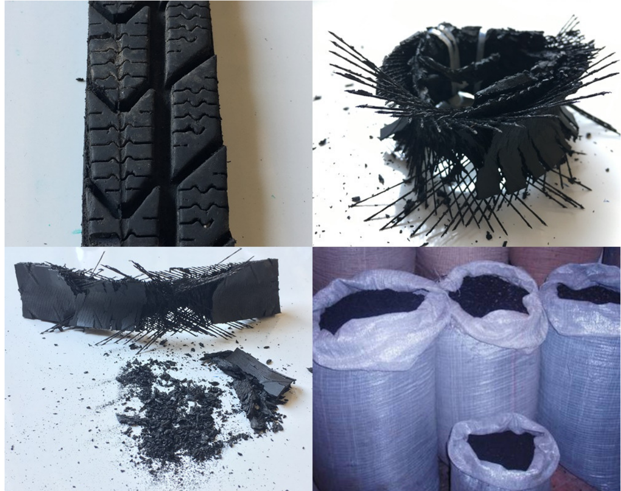
Figure 6. Tire decomposition with Re-Tyre Technology
